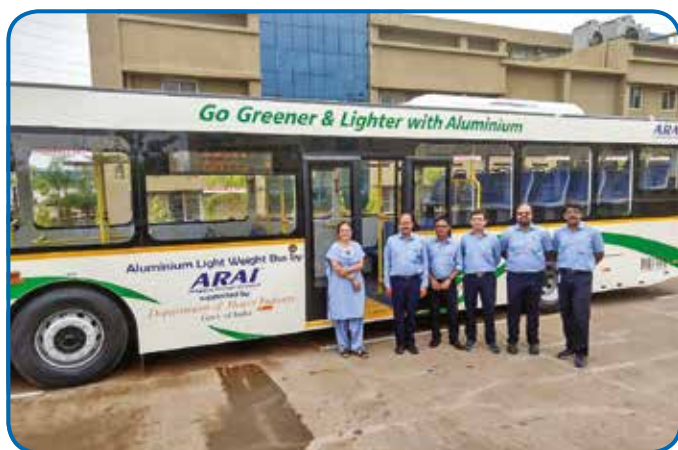
Prototype of Low Floor Bus with Aluminium Superstructure
