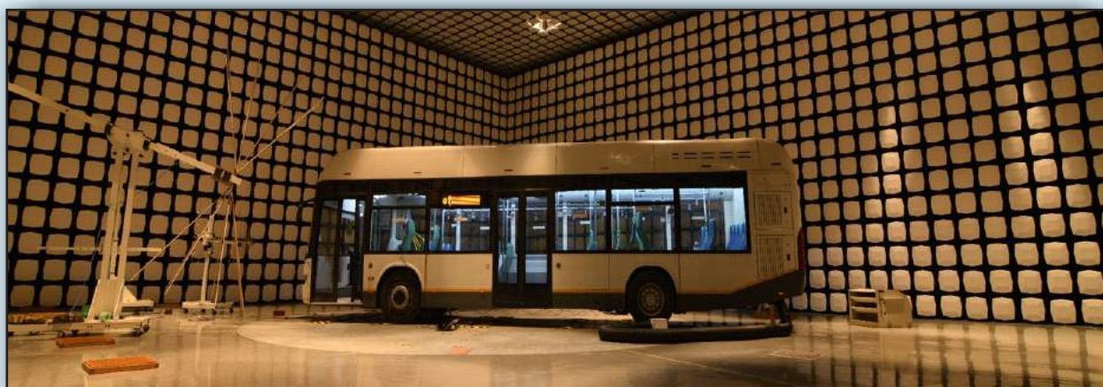
EMC FACILITY AT ICAT
